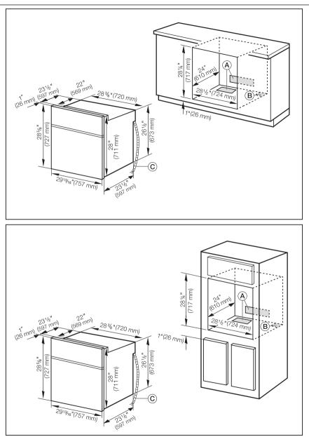
(a) Vent cut-out (min. 24"  $^2$  / 150 cm<sup>2</sup>) possible at rear **or** platform of cabinet (B) Cut-out for power cord (min. 1"  $^2$  / 3 cm<sup>2</sup>)
